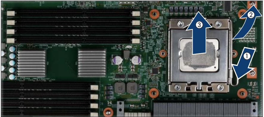
Figure 123: Removing the processor
